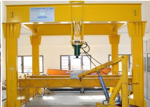
Loading Frame with a capacity of 50 tones
