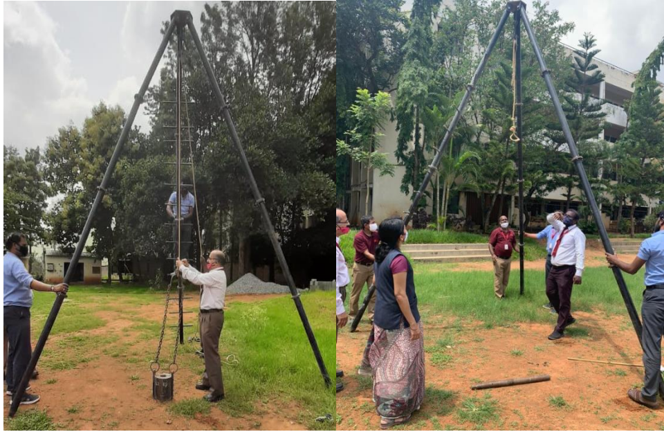
Standard Penetration Test: 63.5 kg - IS -2131:1963
