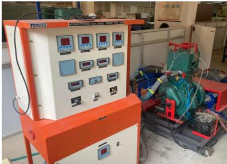
Computerized VCR Diesel Engine Test Rig in Energy conversion Lab
