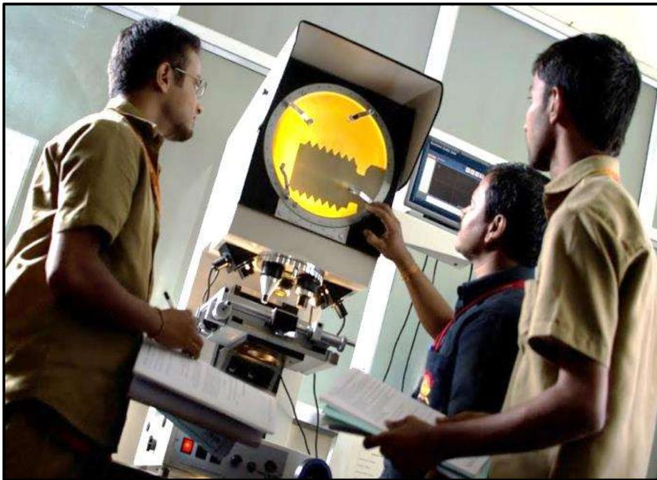
Profile Projector in the Instrumentation and Measurement Lab
